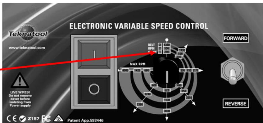
The speed range is achieved with a Variable Speed Controller. A micro-processor chip, in conjunction with other electronic components, allows the input power to be manipulated. In return, smooth Variable DC power can be delivered from the controller to the motor.
