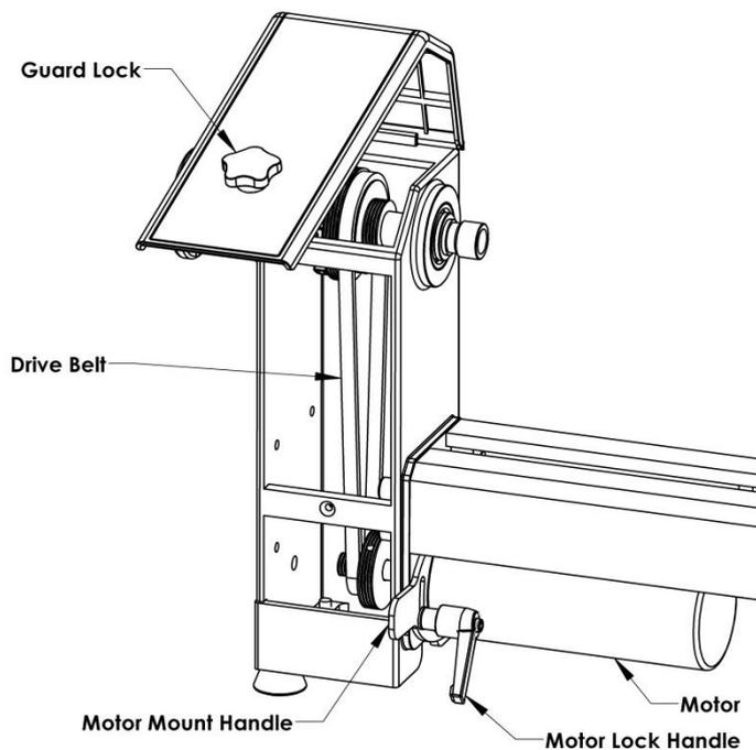
6. Tension the belt by pressing down on the Motor Mount Handle. Pressing down with 2 fingers or the thumb will provide adequate pressure. Slightly higher pressure may be required for larger work.
