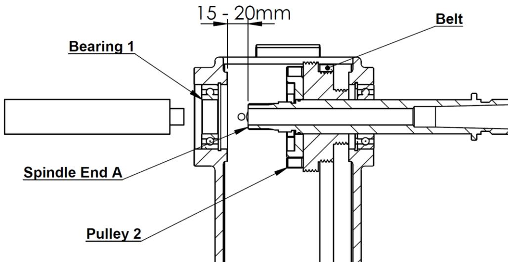
7. Remove the old belt and place the new belt over the **Spindle End A** and on to **Pulley 2**.
