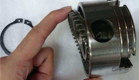
A hand is shown tipping the chuck body over, and the scroll ring is seen falling out from the side.                           |
