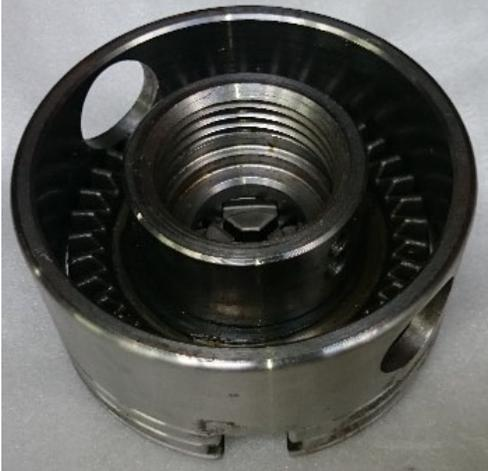
A top-down view of the NOVA G3 chuck with its face down. The central threaded hole and the surrounding jaw slides are visible. |
